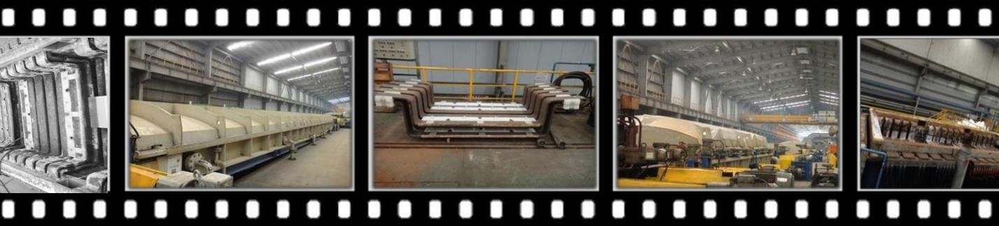
Along with increasing temperature of the acid bath, this process removes impurities, such as scale, rust and stains resulting in high productivity and uniformity in steel strip surface quality. This important process enhances the naturally self-passivate ability of stainless steel.
