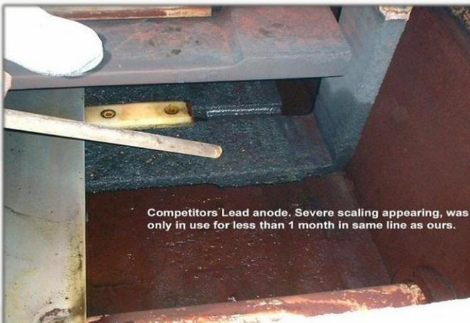
The picture in the left shows a Lead anode made by our competitors. Please check the circled area. It shows a severe scale appearance on the bottom of the anode. It only took less than one month to have serious erosion on this Lead anode.
